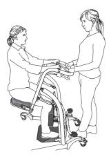
The patient will then be able to sit during transfer. For optimal sitting comfort, the caregiver can regulate the angle of the seat using the adjustment bar on the handlebar. This function also facilitates standing, since the sitting height is higher and the patient's legs are straighter.
