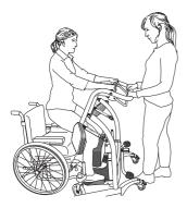
Place the VanMove as close to the patient as possible and ask the patient to place his or her feet on the footrest. Adjust both the height and depth of the leg supports, as well as the seat depth, if necessary.
